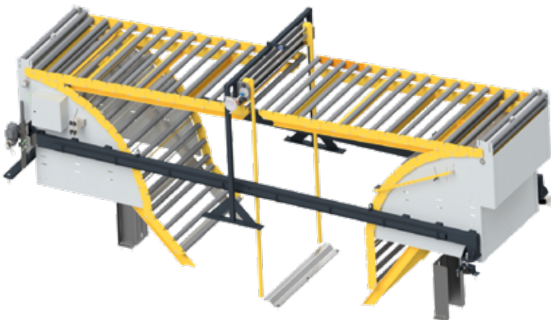
Strip transfer with laser control
